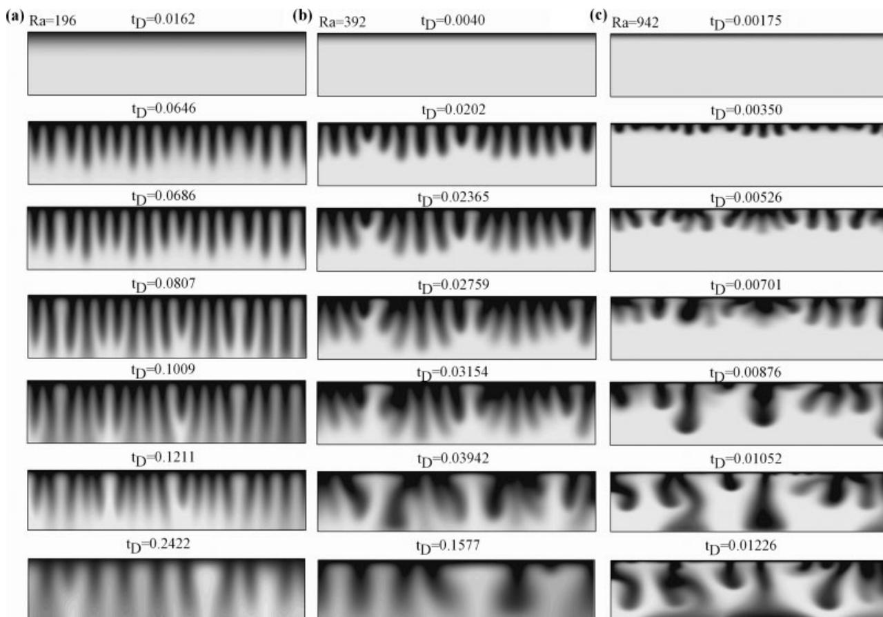
**Figure 5. Evolution of convective mixing fingers for three cases with (a)  $Ra = 196$ , (b)  $Ra = 392$ , and (c)  $Ra = 942$  at different periods of mixing, where darker color means higher concentration.**
