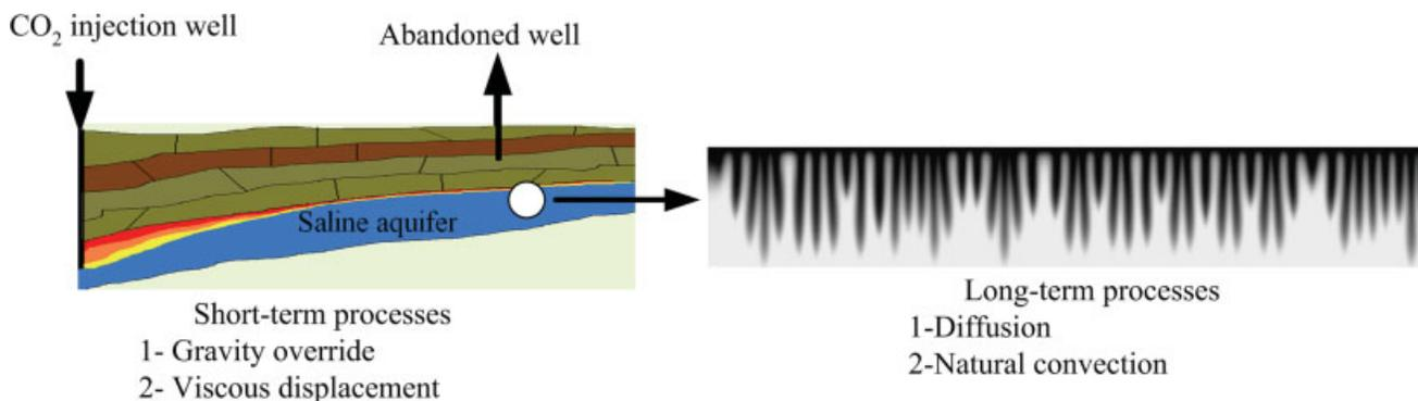
**Figure 1. A schematic of CO<sub>2</sub> injection into a deep saline aquifer describing some of the short-term and long-term processes involved in geological storage of CO<sub>2</sub>.**
