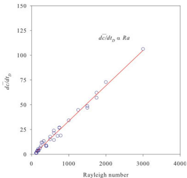
**Figure 4. Dimensionless rate of mixing of CO<sub>2</sub> as a function of Rayleigh number during early stage of the second period of mixing (period B).**
