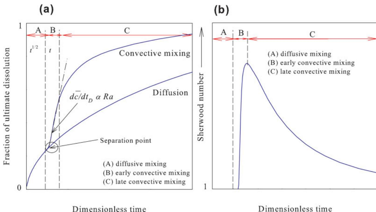
**Figure 3. Typical dissolution (a) and Sherwood number (b) curves for convective mixing.**
