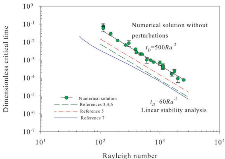
**Figure 7. Onset of convection as a function of Rayleigh number obtained from numerical simulations as compared with linear stability analysis.<sup>3-7</sup>**
