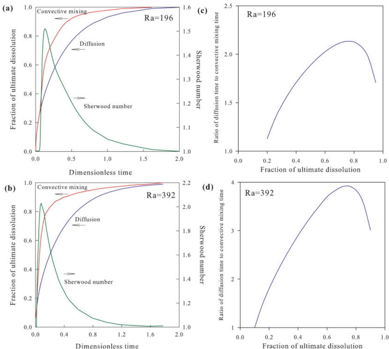
**Figure 6.** Dissolution and Sherwood number curves for two cases with (a)  $Ra = 196$  and (b)  $Ra = 392$  as a function of dimensionless time; the ratio of diffusion time to convective mixing time as a function of dissolution for the two Rayleigh numbers is shown on the right (c,d).
